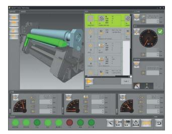
The 3D operator interface of the plate bending machines allows intuitive and convenient operation of the machine.
